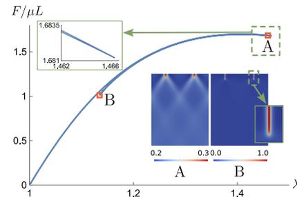
FIG. 6. Normalized axial force  $F/\mu L$  versus the mean stretch  $\lambda$  for the near wrinkling case ( $H/L = 2.5$ ). The insets on the right show the distribution of the internal variable  $\alpha$  in the reference configuration corresponding to the points A and B. The parameter  $\ell_0/H = 0.01$ .
