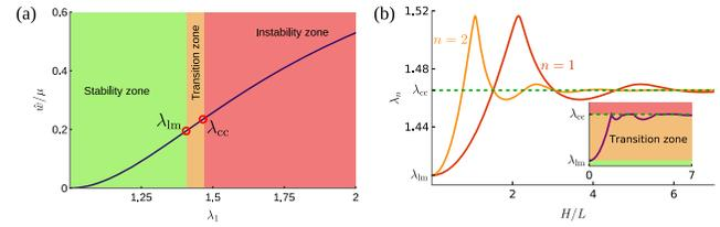
FIG. 2. (a) The energy density  $\hat{w}(\lambda)$  of our softening material as a function of the maximal principal stretch  $\lambda_1$ . (b) The stability curves for the two modes with  $n = 1, 2$ ; the purple line in the inset represents the function  $\lambda_{\text{cr}}(H/L)$ .
