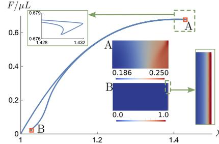
FIG. 5. Normalized axial force  $F/\mu L$  versus the mean stretch  $\lambda$  for the near necking case ( $H/L = 1$ ). The insets on the right show the distribution of the internal variable  $\alpha$  in the reference configuration corresponding to the points A and B. The parameter  $\ell_0/H = 0.01$ .
