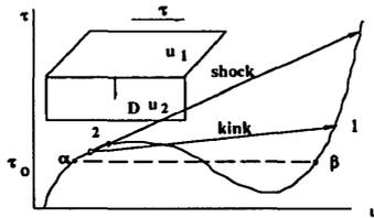
Figure 1. A typical isotherm  $\tau = \tau(u, T = \text{const})$  for the solid which allows for martensitic phase transformation.
