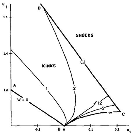
Figure 2. The deformation ( $u_1/\Delta u$ ) of the state behind the martensitic phase boundary, as a function of the deformation ( $u_2/\Delta u$ ) of the state in front of it. CJ regimes are sonic with respect to the state in front.
