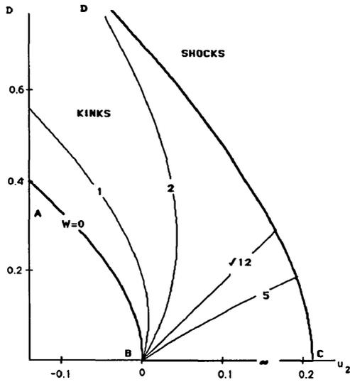
Figure 3. Phase boundary velocity ( $D/\sqrt{K\Delta u}$ ) as a function of the state of deformation ahead of it ( $u_2/\Delta u$ ) for different values of the non-dimensional parameter  $W$ .
