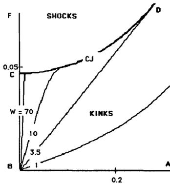
Figure 4. Kinetic laws, following from the exact solution for a different  $W$ ; here  $F$  is the "driving force" measuring the degree of the metastability while  $D$  is the conjugate mass flux.
