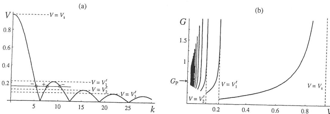
Figure 5.2. (a) Real wave numbers  $k$  corresponding to a given interface velocity  $V$  with “+” and “-” denoting the sign of  $kL'(k)$ . Also marked are the resonance velocities  $V_i^r$ . (b) Mobility curves  $G(V)$ . The entire region around the resonances should be excluded. In both graphs  $\beta = -1/8$ .
