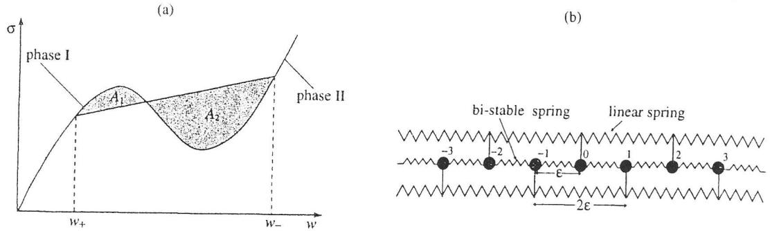
Figure 5.1. (a) The macroscopic stress-strain law and the Rayleigh line for a subsonic phase boundary. The difference  $A_2 - A_1$  between the shaded areas is the configurational force  $G$ . (b) The discrete microstructure with nearest and next-to-nearest neighbor interactions.
