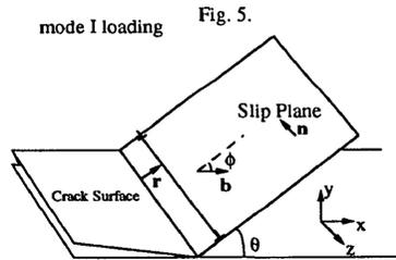
Fig. 5. The crack system with crack surfaces of normal *y* and crack front *z*, slip system with slip plane normal *n* and slip vector *b*; the crack is under mode I loading.
