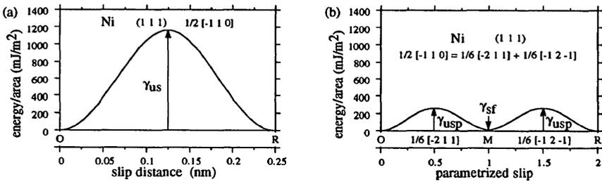
Fig. 2. The energy of a generalized stacking fault on (111) plane in Ni as a function of the slip distance in the straight route Fig. 2a and the partial route Fig. 2b.
