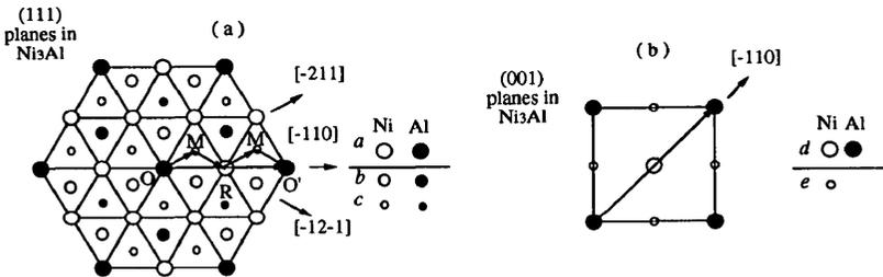
Fig. 1. The  $\text{Ni}_3\text{Al}$  (111) (Fig. 1a) and (001) (Fig. 1b) planes. Open and filled circles represent the Ni and Al atoms. Large, medium, and small circles in Fig. 1a represent the  $a$ ,  $b$ , and  $c$  planes layers, respectively. Large and small circles in Fig. 1b represent the  $d$  and  $e$  layers, respectively.
