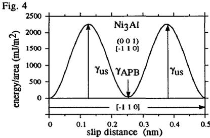
Fig. 4. The energy of a generalized stacking fault on (001) plane in Ni<sub>3</sub>Al as a function of the slip distance in the straight route.
