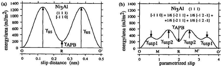
Fig. 3. The energy of a generalized stacking fault on (111) plane in  $\text{Ni}_3\text{Al}$  as a function of the slip distance in the straight route Fig. 3a and the partial route Fig. 3b.
