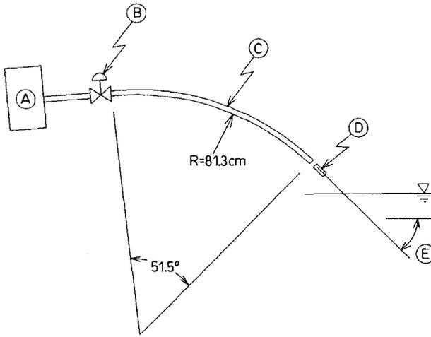
Fig. 1. Sphere propulsion apparatus. A air reservoir; B solenoid actuated valve; C polyethylene tube; D sphere speed measurement device; E adjustable angle,  $30^\circ$  to  $45^\circ$
