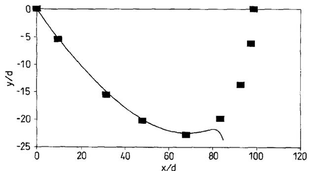
Fig. 4. Sphere trajectory for Run A compared with the analysis, assuming constant  $C_L$
