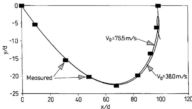
Fig. 6. Effect of initial velocity  $V_0$  on sphere trajectory for Run A with  $C_L = 0.037/V$  and  $C_D = 0.075$ . The curve for  $V_0 = 150 \text{ m/s}$  coincides with that for  $V_0 = 76.5 \text{ m/s}$
