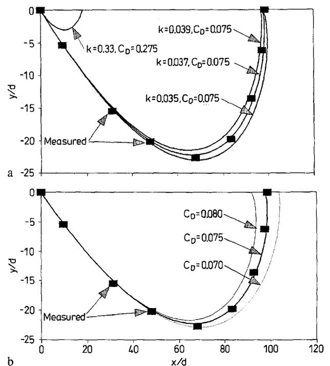
Fig. 3a, b. Sphere trajectory for Run A (76.5 m/s at  $30^\circ$  incident angle) compared with analysis assuming  $C_L=k/V$ . a Effect of varying  $k$ ; b effect of changes in  $C_D$
