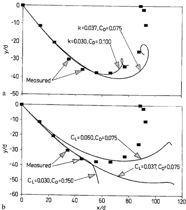
Fig. 5a, b. Sphere trajectory for Run B (81.9 m/s at  $45^\circ$  incident angle) compared with analysis. a Analysis assuming  $C_L = k/V$ ; b assumes constant  $C_L$
