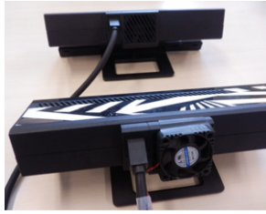
Fig. 2. Detail and general specifications of the fan used as external cooling system.
