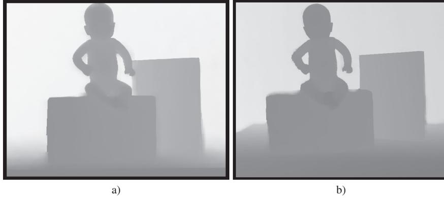
Fig. 5.8 Bilateral upsampling of depth data from a ToF camera (a) and from Kinect<sup>TM</sup> (b).
