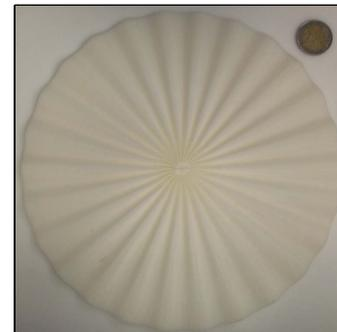
**Fig. 6.** Photograph of the experimental model produced with the rapid prototyping technique. In the right top of the figure, a 2-euro coin is shown for size comparison.
