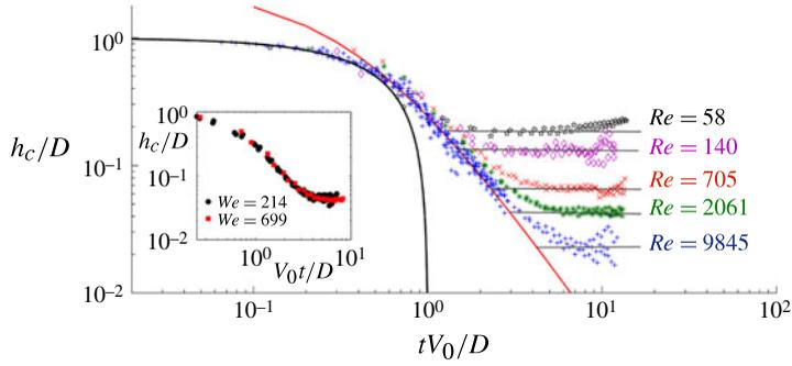
FIGURE 5. (Colour online) Logarithmic plot of the evolution of  $h_c$  with time for different Reynolds numbers and similar Weber numbers  $(Re, We) = (9845, 382), (2061, 467), (705, 479), (140, 449)$  and  $(58, 539)$  respectively. Black solid line, ballistic regime; red dotted line, self-similar regime; black dotted lines, plateau regime ( $h_p$ ). The inset shows the evolution of  $h_c$  in time for similar Reynolds numbers but different Weber numbers (2690, 214) and (2440, 699).
