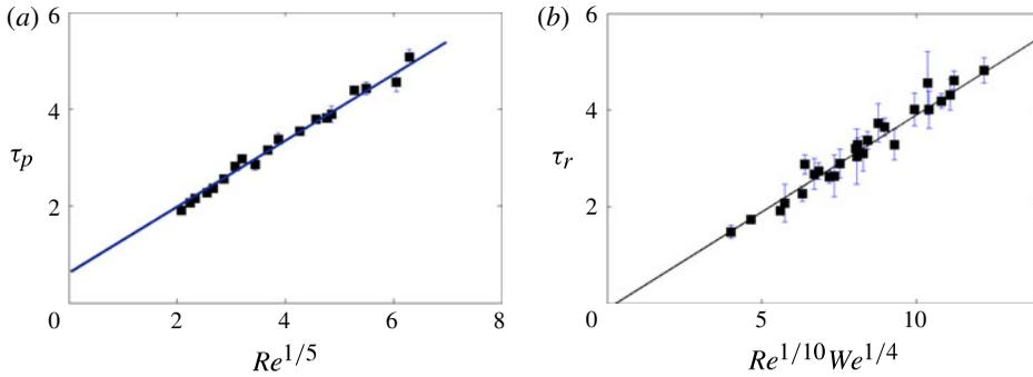
FIGURE 7. (Colour online) (a) Dimensionless cross-over time  $\tau_p = V_0 t_p / D$  between inertial and viscous regimes in the central layer as a function of  $Re^{1/5}$ . (b) Dimensionless time of the maximal radial expansion  $\tau_r$  as a function of  $Re^{1/10} We^{1/4}$ .
