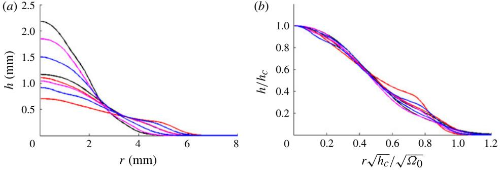
FIGURE 4. (Colour online) (a) Series of drop profiles at times 1.14, 1.25, 1.34, 1.5, 1.52, 1.62, 1.71 and 1.87 in the non-dimensionalized time unit for  $We = 255$  and  $Re = 1470$ , each colour corresponding to one experiment. (b) Collapse of the same profiles using the self-similar variables  $h/h_c$  and  $r\sqrt{h_c}/\sqrt{\Omega_0}$ , with  $h_c$  the height of the centre of the drop and  $\Omega_0$  its volume.
