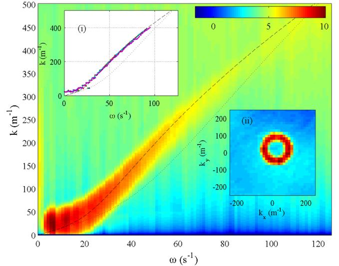
FIG. 4 (color online). Experiments II: Typical spectrum  $|\eta_{k,\omega}|^2$  at forcing amplitude  $A = 20$  mm. Inset (i) shows the collected dispersion relations for  $A = 1, 6, 12, 20,$  and  $28$  mm. The dashed line shows the linear dispersion relation and the dotted line the first nonlinear mode. Inset (ii) illustrates the isotropy in the  $(k_x, k_y)$  space by plotting  $|\eta_{k,\omega}|^2$  for  $\omega = 27.64$  s $^{-1}$ .
