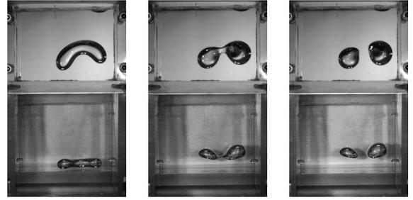
**Fig. 6.** Bubble at the moment of breakup in the middle of the cell in  $\mu G$  ( $A = 4.2$  cm and  $f = 1.3$  Hz with silicone oil of  $0.5$  cm<sup>2</sup>/s). In each picture, the upper and lower half is in longitudinal and transversal view, respectively.
