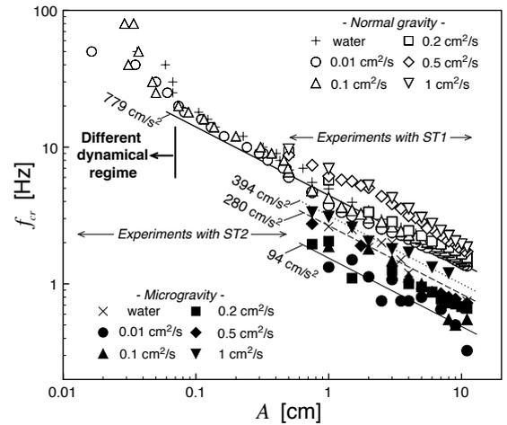
**Fig. 7.** Critical frequency of bubble breakups in micro- and normal-gravity environments. Bubble volume is  $3$  cm<sup>3</sup> for all the data. Curves of constant acceleration are also shown for the values discussed in the text.
