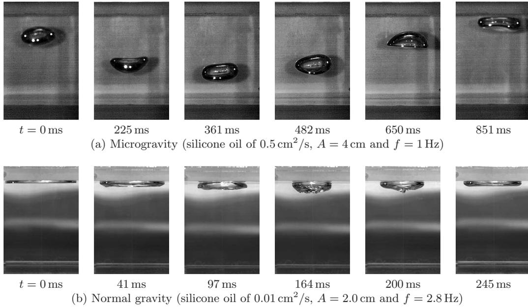
**Fig. 2.** Side views of bubble motion under an oscillatory acceleration field.
