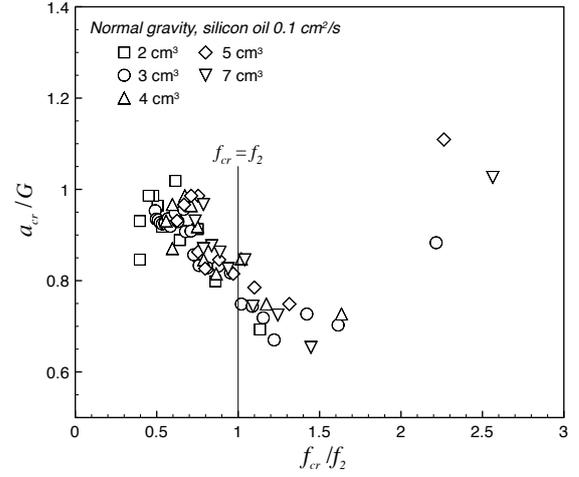
**Fig. 9.** Dimensionless critical acceleration for the breakups of a bubble of  $3 \text{ cm}^3$  in silicone oil of viscosity  $0.1 \text{ cm}^2/\text{s}$ . The bubbles of volumes  $V_b = 2, 3, 4, 5$  and  $7 \text{ cm}^3$  have natural frequencies  $f_2$  of  $3.66, 2.99, 2.60, 2.32$  and  $1.97 \text{ Hz}$ , respectively.
