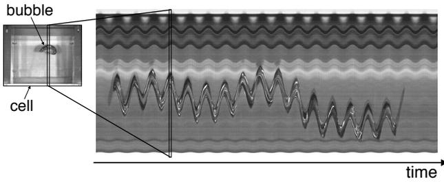
**Fig. 3.** Space-time diagram of bubble motion (the right larger image) in transversal view in  $\mu G$ . The suspending liquid is silicone oil of  $0.5 \text{ cm}^2/\text{s}$  and the oscillation parameters are  $A = 1.5 \text{ cm}$  and  $f = 1.6 \text{ Hz}$ . The left smaller image shows how the diagram is constructed (see the text for details).
