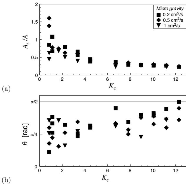
**Fig. 4.** Amplitude and phase of bubble motion in  $\mu G$ .
