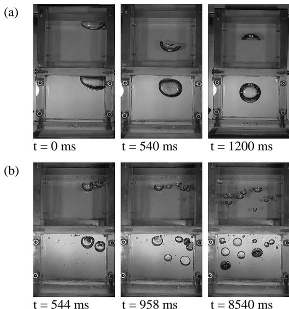
Fig. 1: Bubbles under vibrations (a) with no break-up (silicon oil 47V50,  $f=0.8$  Hz,  $A=7.0$  cm) and (b) with break-up (silicon oil 47V100,  $f=2.5$  Hz,  $A=6.0$  cm).  $t=0$  corresponds to the start of vibrations. In each picture, the upper half part represents a side view obtained by reflection on the mirror and the lower half corresponds to a view along the vibration axis.
