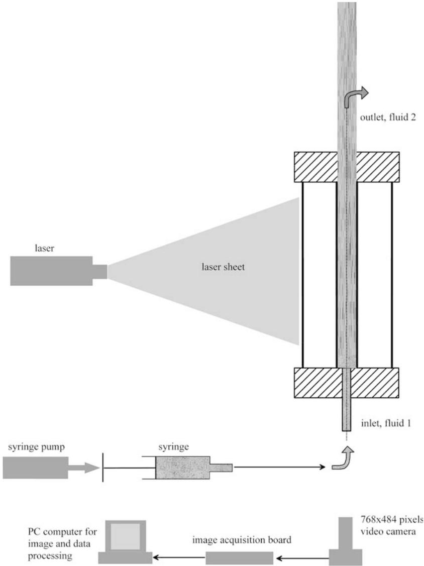
**Fig. 1.** Schematic diagram of the experimental setup for DPIV measurement of a more viscous fluid 2 displaced by a less viscous fluid 1 in a vertical cylindrical tube
