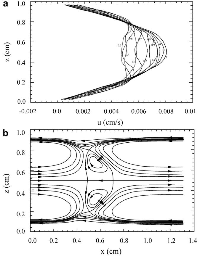
Fig. 6a, b. The velocity field around the fingertip of a downward displacement of 100cs into 1000cs silicone oil in a tube of 1 cm diameter with  $Pe = 9 \times 10^4$ . (a) Velocity profiles with  $x$  location of each profile numbered, and (b) streamline pattern with a zero streamline (finger profile) highlighted
