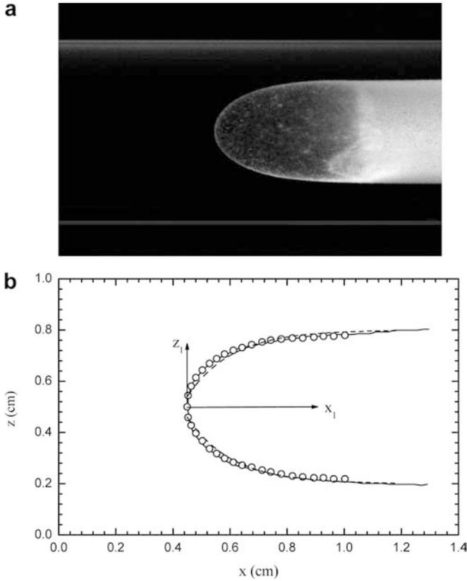
Fig. 5a, b. Finger profile of an upward displacement (a) image profile and (b) finger profile from zero streamline in Fig. 4d. The dashed line is a fitting of zero streamline using Eq. 3
