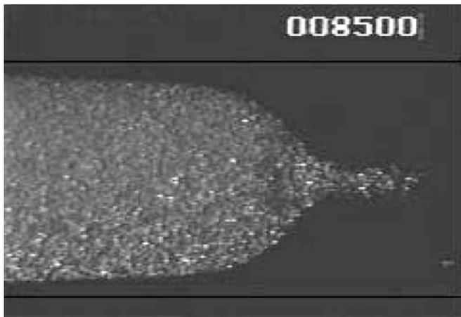
Fig. 7. Image of a spike on the fingertip for downward displacement of 100cs into 1000cs silicone oil in a tube of 1 cm diameter at  $Pe=9\times 10^4$
