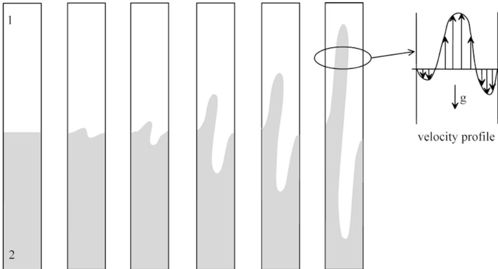
**Fig. 2.** Sketch of a finger evolution from an unstable interface with no flow injection
