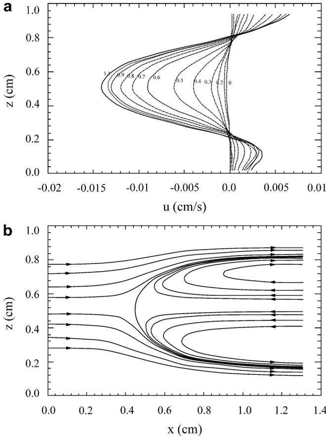
Fig. 3a, b. The velocity field around the fingertip of an upward displacement in a tube of 1 cm diameter with no fluid injection. (a) Velocity profiles with  $x$  location of each profile numbered. (b) Streamline pattern with the zero streamline highlighted
