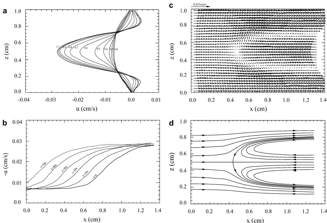
**Fig. 4a–d.** The velocity field around the fingertip of an upward displacement of 100cs into 1000cs silicone oil in a tube of 1 cm diameter with  $Pe=7.7\times 10^4$ . (a) Velocity profiles with  $x$  location of each profile numbered. (b) Velocity distributions along the tube
