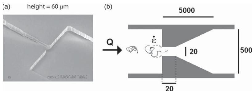
**Fig. 2.** (a) MEB picture of the constriction. (b) Schematic projection of the planar  $60 \mu\text{m}$  high constriction. Dimensions are indicated in microns. The dotted circle line delimits the zone of strong elongation.
