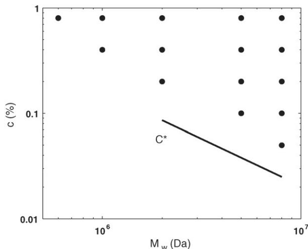
Fig. 1. Mass and concentration diagram of the aqueous PEO solutions.
