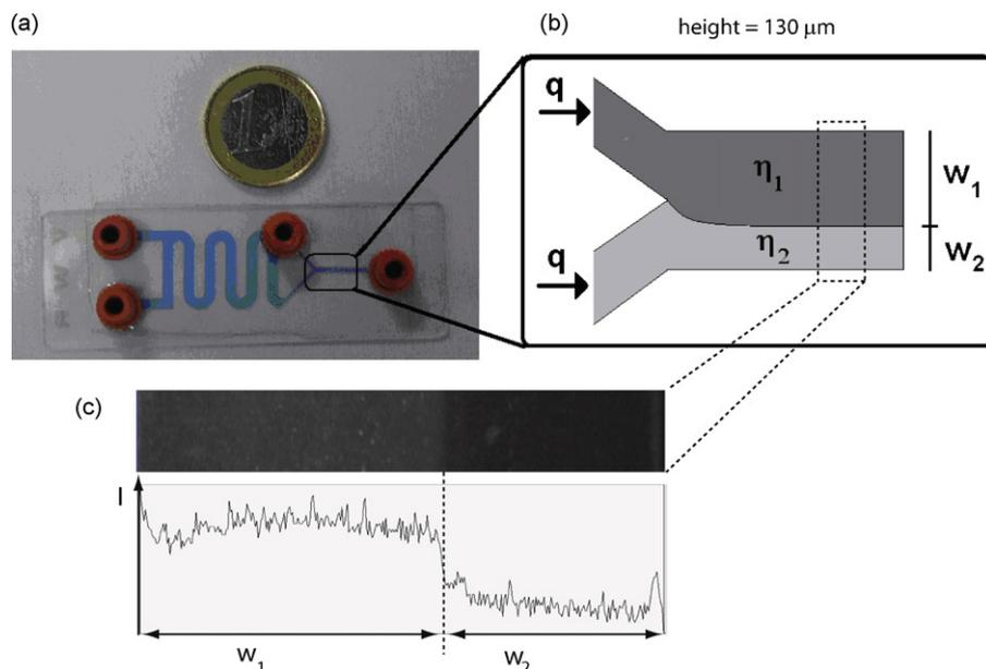
**Fig. 3.** (a) Picture of the chip with its connectors, the serpentine reservoir and the viscosimeter. (b) Schematic focus on the viscosimeter and its principle. (c) Experimental image of the interface and fluorescence intensity profile along the width from which the interface position is determined.
