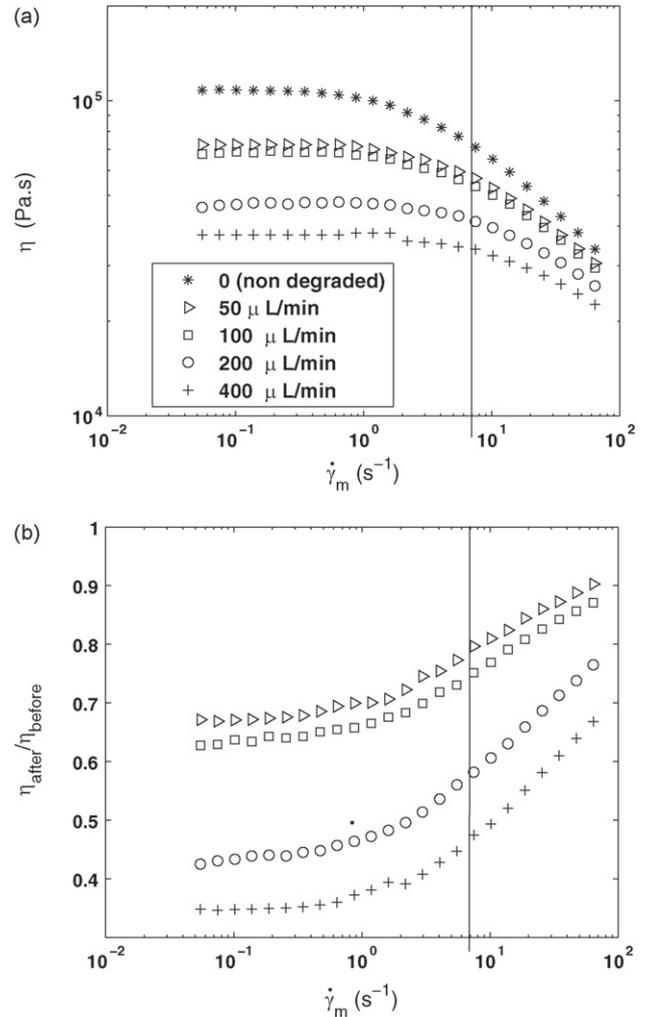
**Fig. 6.** (a) Viscosity curves measured in a Low-shear 30 rheometer of non-degraded and degraded 0.4% 5 MDa PEO solutions prepared in the constriction at different flow rates (in  $\mu\text{L}/\text{min}$ ): 0 (\*), 50 (triangles), 100 (squares), 200 (o), 400 (+). The vertical line indicates the shear rate at which viscosity ratio is measured inside the microfluidic viscosimeter. (b) Ratio between the viscosity before and after degradation.
