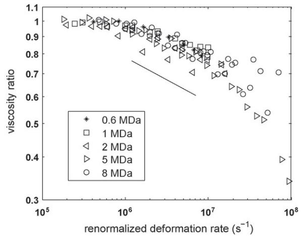
**Fig. 12.** Viscosity loss curves versus a renormalized imposed deformation rate  $\dot{\gamma}_d \times (M_w/M_0)^{-1.7} (c/c_0)^{0.7}$ . This collapse is obtained for all the solutions prepared with the characteristics represented in Fig. 1. For a given mass, the different concentrations are represented by a same symbol. The straight line indicates the mean slope obtained from the viscosity decay fit as represented on the few solutions of Fig. 8.
