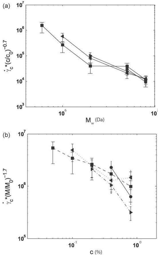
**Fig. 11.** (a) Mass dependence of the critical deformation rate  $\dot{\gamma}_c$  rescaled by its concentration power law dependence. (b) Concentration dependence of the critical deformation rate  $\dot{\gamma}_c$  rescaled by its mass power law dependence.
