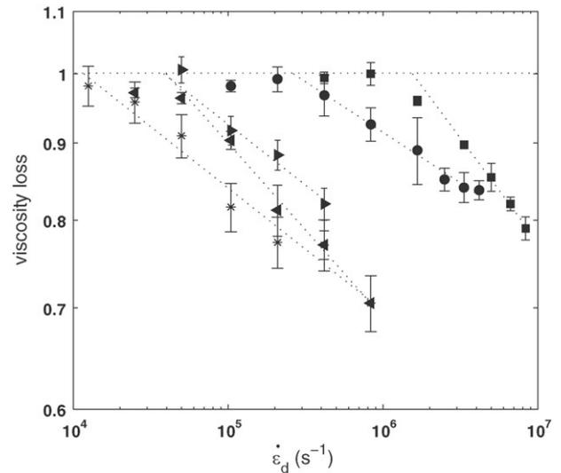
**Fig. 9.** Viscosity loss of 0.8% PEO solutions of varying mass: 8, 5, 2, 1 and 0.6 MDa with the linear fit of the points representing a significant viscosity loss. For clarity reasons, only the solutions corresponding to the five top points in Fig. 1 have been represented.
