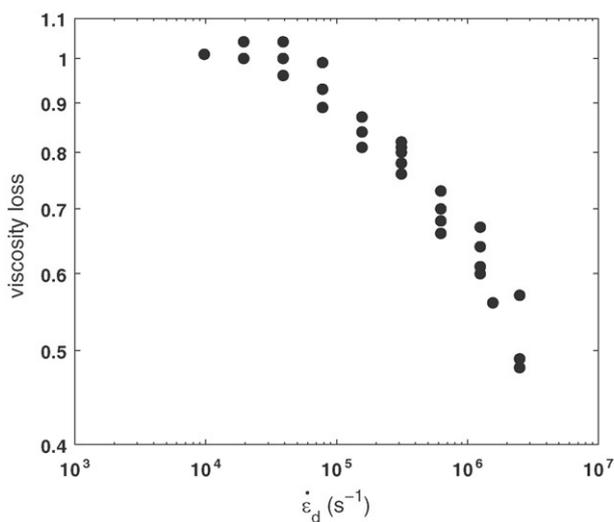
**Fig. 8.** Viscosity ratio measured in the chip at  $\dot{\gamma}_m = 5.5 \text{ s}^{-1}$  versus the maximum imposed deformation rate  $\dot{\varepsilon}_d$  for a 0.4% 5 MDa PEO solution.
