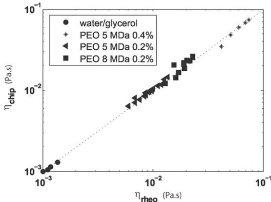
**Fig. 7.** Comparison between the viscosity measured in a Low-shear 30 rheometer and measured in the chip for water and glycerol mixtures and 3 different PEO solutions degraded at different flow rates. For each point, the measurement shear rate in the Couette rheometer  $\dot{\gamma}_r$  equals the measurement shear rate at the wall of the chip viscosimeter  $\dot{\gamma}_m$ . For the polymer solutions, measurement shear rates have been varied between 5.5 and 63.9  $\text{s}^{-1}$ .
