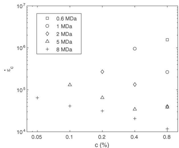
**Fig. 10.** Critical deformation rate  $\dot{\varepsilon}_c$  for degradation versus concentration for different polymer average molecular weights.
