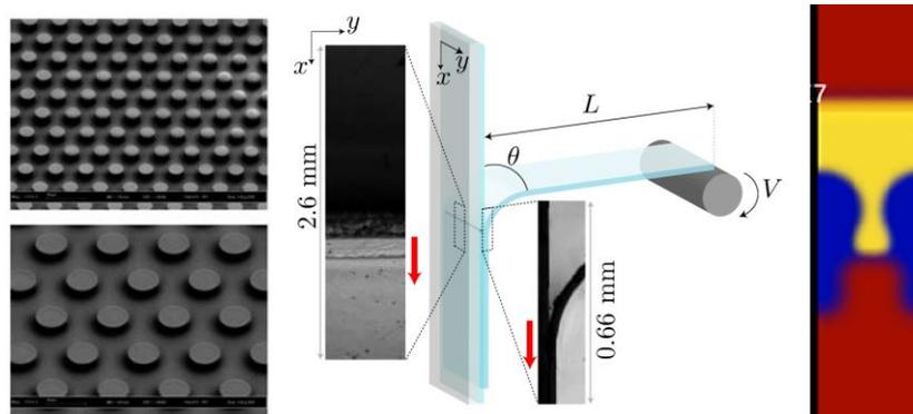
*Left: Micro-patterned substrates. Middle: Peeling experiment. Right: Simulation of adhesive detachment from a pillar*
