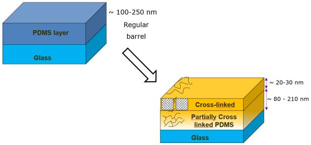
Figure 1: Structure of the cross-linked silicone
