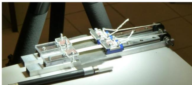
Figure 1: (left) Edge of a clay film of thickness of about 50  $\mu\text{m}$  observed by ESEM and (right) 2 clays films in a device enabling mechanical solicitation for creep experiments. Figures from Carrier's Ph.D. thesis (2013).
