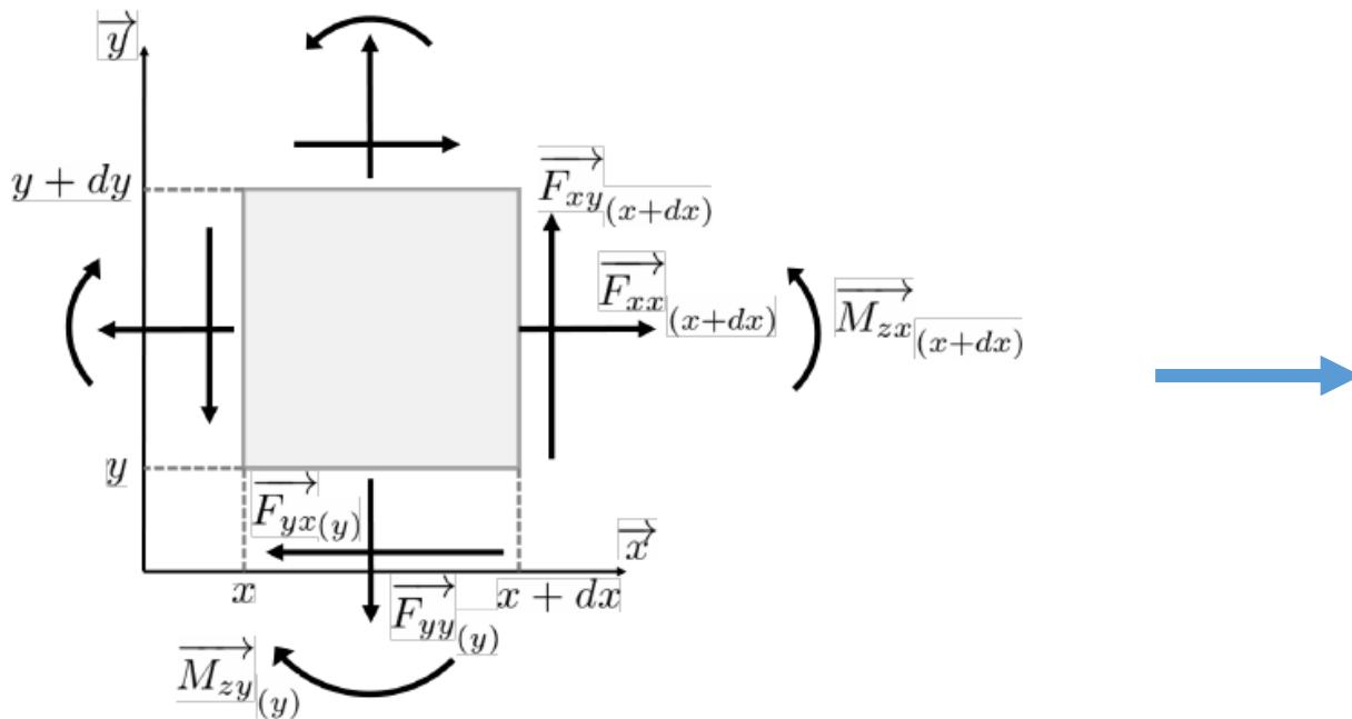
$$\begin{aligned} \mathbf{div}(\boldsymbol{\sigma}) &= \rho \ddot{\mathbf{u}} \\ \mathbf{div}(\mathbf{m}) - (\sigma_{xy} - \sigma_{yx}) &= I \ddot{\theta} \end{aligned}$$
