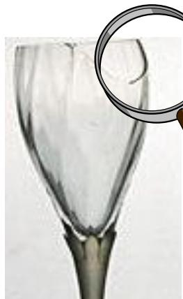
[here Silica glass broken upon stress corrosion]
