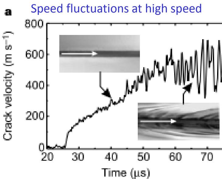
Transition to mist/hackle fracture surface at high speed
