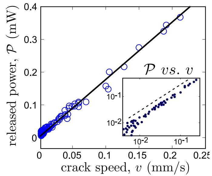
Proportionality between  $P$  and  $v$  → Material constant  $\Gamma \sim 100 \text{ J/m}^2$
