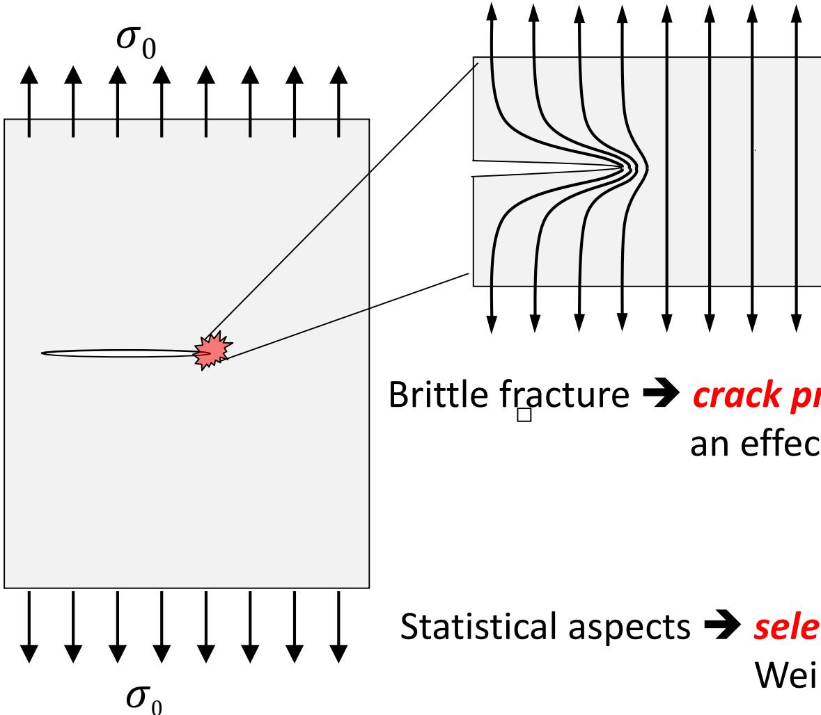
Brittle fracture → ***crack propagation problem*** into an effective homogeneous medium
