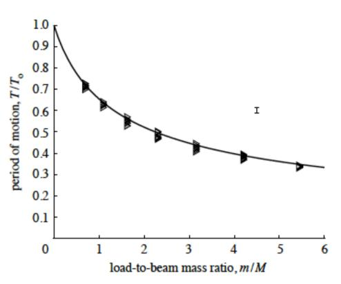
mensionless period of load motion versus load-to-beam mass ratio for loads released near of an initially horizontal beam,  $|x_0/L - 0.5| \le 0.25$ . The triangles denote the y observed periods. The theoretically predicted period is given by the solid curve and 19). A characteristic error bar is shown.  $\mathcal{K}=0.744$ ,  $\theta=0$ ,  $T_0=(4\pi/15)\sqrt{630}\sqrt{EI/Mg^2L}$ .
