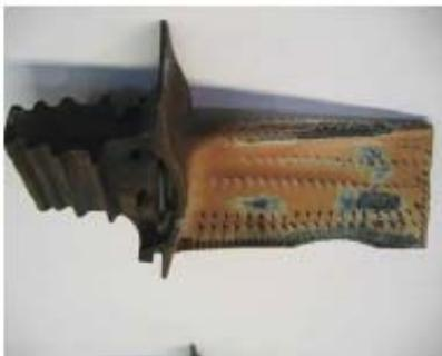
Blade showing spalled TBC
