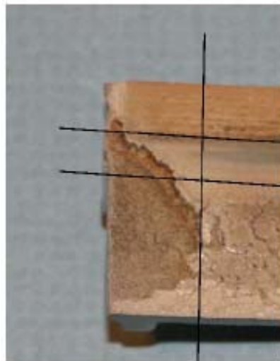
Spalled region under CMAS
