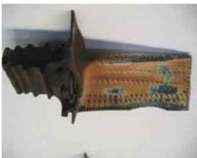
Blade showing spalled TBC
