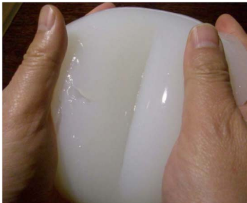
Crease on the surface on a starch-gel from Hong, Zhao and Suo (2009).
