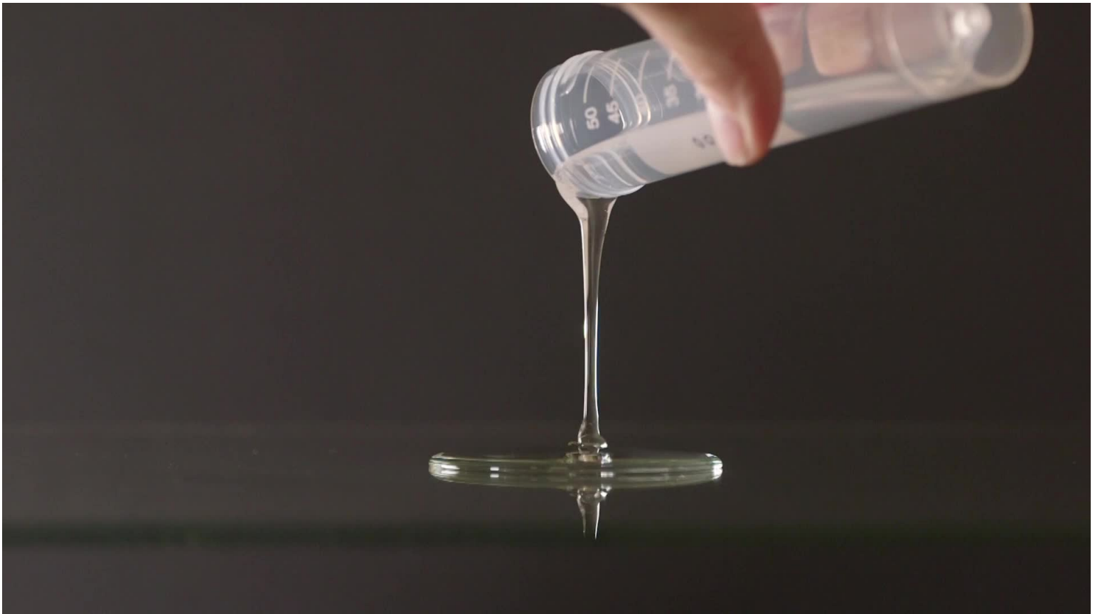
Figure 1. Rayleigh–Taylor Instability in a thin viscous film (Experiment : Christophe Clanet)
