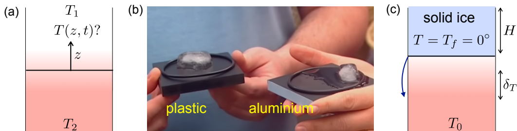
Figure 1: a. A pair of semi-infinite solids of different initial temperatures are brought in contact. What sets the temperature at the interface? b. Ice cube melting faster on a block of Aluminium than on a block of plastic (or wood). Image from Veritasium YouTube channel https://youtu.be/vqDbMEdLiCs . c. Simplified model. An ice cube of initial temperature T = T_f = 0^\circ\text{C} sits on a semi-infinite solid of initial room temperature T_1 = 20^\circ\text{C} . We assume that the water formed by melting the ice immediately flows away leaving the remaining ice cube in contact with the solid.
