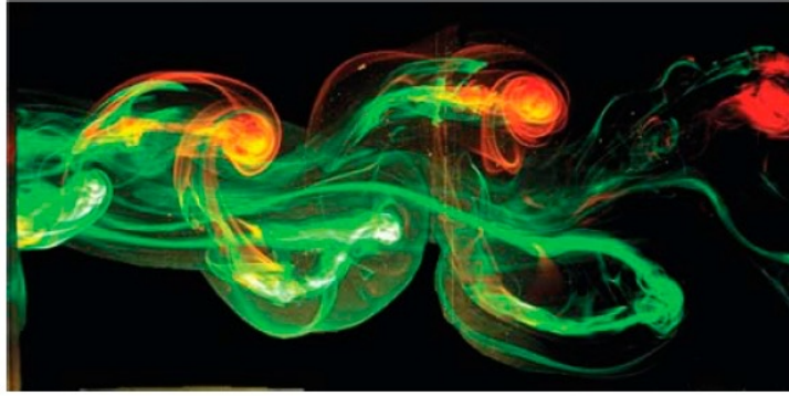
FIGURE 8. Flow visualization in the near wake of the fin at \phi = 90^\circ and St_A = 0.15 . The green dye was injected from one side of the fin, the red dye from the other side. Flow is from left to right. View is from above, looking along the span.
