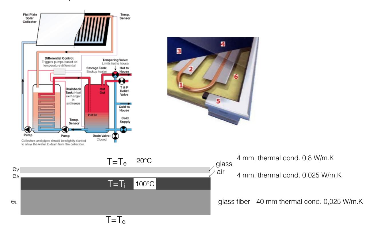
use the 1D steady state diffusion and the concept of thermal resistance to compute heat fluxes on both sides of the collector
