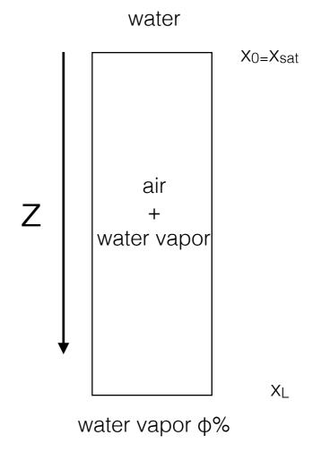
Write the molar fluxes of vapor  $N_A$  and air  $N_B$  as a function of molar fractions  $x_A$  and  $x_B$
