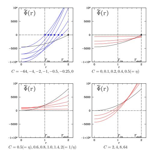
The figure above shows  $\tilde{\Phi}(r) \equiv 4r^2\Phi(r)$  for  $\eta = 0.5$ . We set  $Re_{\rm in}^2 + Re_{\rm out}^2 = 100^2$  and scan over positive and negative values of C.
