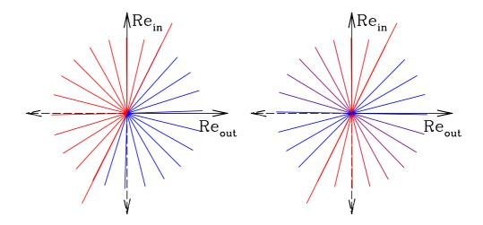
The figure on the left illustrates a change in stability at the Rayleigh line, which does not respect the physically necessary centro-symmetry of the  $(Re_{\text{out}}, Re_{\text{in}})$  plane. Red is used to denote the unstable parameters and blue the stable parameters.
