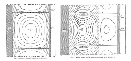
The figure above shows sketches of flow in the corotating and counter-rotating regimes Taylor's famous 1923 paper. The corotating vortices fill up the entire domain, whereas the counter-rotating spiral vortices are localized near the inner cylinder, where  $\Phi$  is negative.
