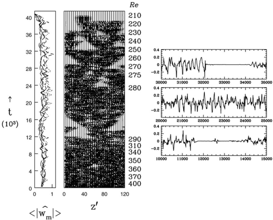
Figure 15. Evolution for  $\theta = 0^\circ$  with  $L_{x'} = L_x = 10$  and  $L_{z'} = L_z = 120$ .  $Re$  is lowered by steps of  $\Delta Re = 5$ ; not all intermediate values of  $Re$  are shown. The flow continues to have turbulent regions far below  $Re = 300$ . Left: evolution over the entire domain, showing the formation and disappearance of turbulent domains. Right: evolution of  $w(x = 0, y = 0, z = 60, t)$ , showing irregular periodic cycles.
