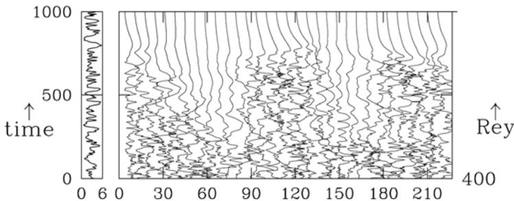
*Figure 14.* Evolution for  $\theta = 90^\circ$ . Two simulations at  $Re = 400$  are shown, in domains with  $L_{x'} = L_{z'} = 4$ . The domain shown on the right has  $L_{z'} = L_x = 220$ ; that on the left has  $L_{z'} = L_x = 6$ , close to the minimal flow unit (the two are not shown to scale). The large domain supports a transient pattern as an intermediate state between uniform turbulence and laminar Couette flow, whereas the turbulence persists in the small domain.
