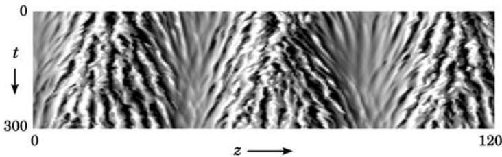
Figure 9. Space-time plot showing dynamics of the turbulent-laminar pattern. Streamwise velocity is sampled along a spanwise cut through the flow field (the line  $x = y = 0$  in the reconstructed flows in Figure 6). Time zero corresponds to the time of Figure 6. The streaks propagate away from the center of the turbulent regions toward the laminar regions.
