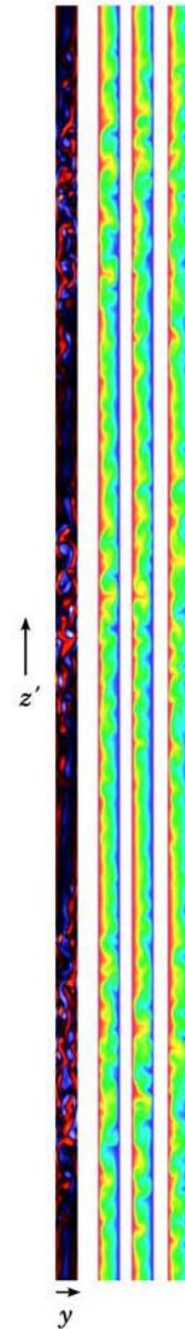
Figure 7. Turbulent-laminar pattern at  $Re = 350$  viewed between the moving plates ( $x' = 0$  plane). Left plot shows streamwise vorticity. The other three plots show contours of streamwise velocity at three times separated by 100 time units (time increasing left to right). The vorticity plot and the first velocity plot correspond to the field seen in Figure 6.
