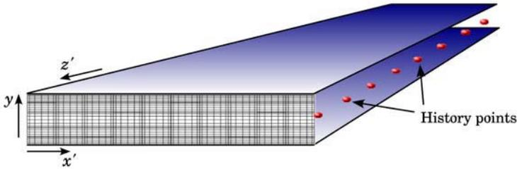
Figure 4. Simulation domain. The  $(x', y)$  grid is the actual spectral-element mesh used for the case  $L_{x'} = 10$ . Only part of the  $z'$  direction is shown. In practice we use 32 history points in the  $z'$  direction.
