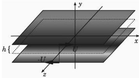
Figure 1. Plane Couette geometry. Plates separated by a gap  $2h$  move at speeds  $\pm U$ . The coordinate system we use is as shown, with  $y = 0$  corresponding to midgap.
