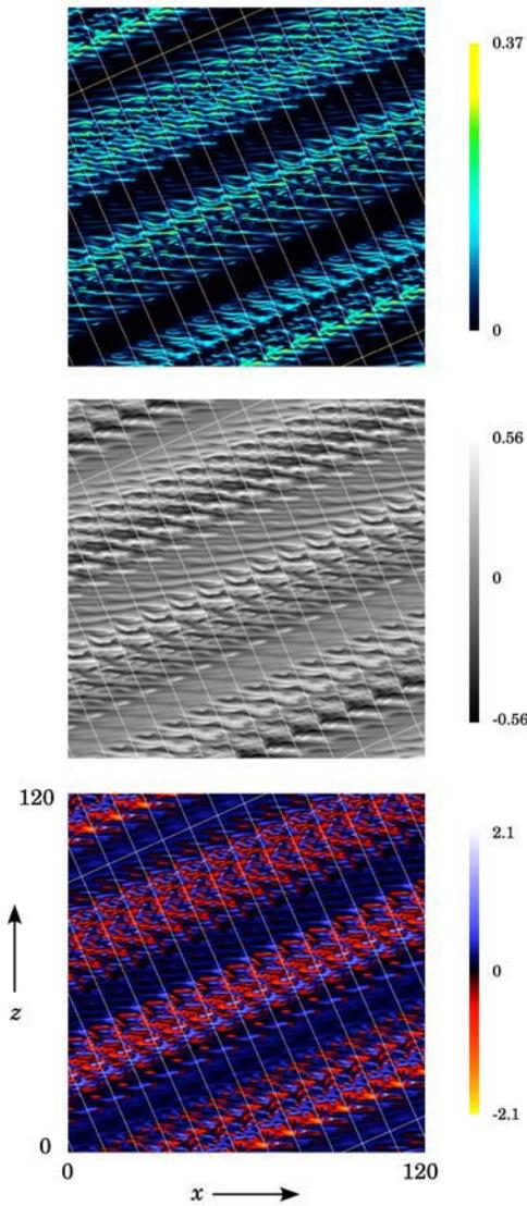
Figure 6. Turbulent-laminar pattern at  $Re = 350$ . The kinetic energy, streamwise velocity, and streamwise vorticity are visualized in the  $y = 0$  plane, midway between and parallel to the moving plates. The computational domain (outlined in white, tilted at angle  $\theta = 24^\circ$ ) is repeated periodically to tile an extended region in  $x$ - $z$  coordinates. Streamwise streaks, with spanwise separation approximately  $4h$ , are visible at the edges of the turbulent regions.
