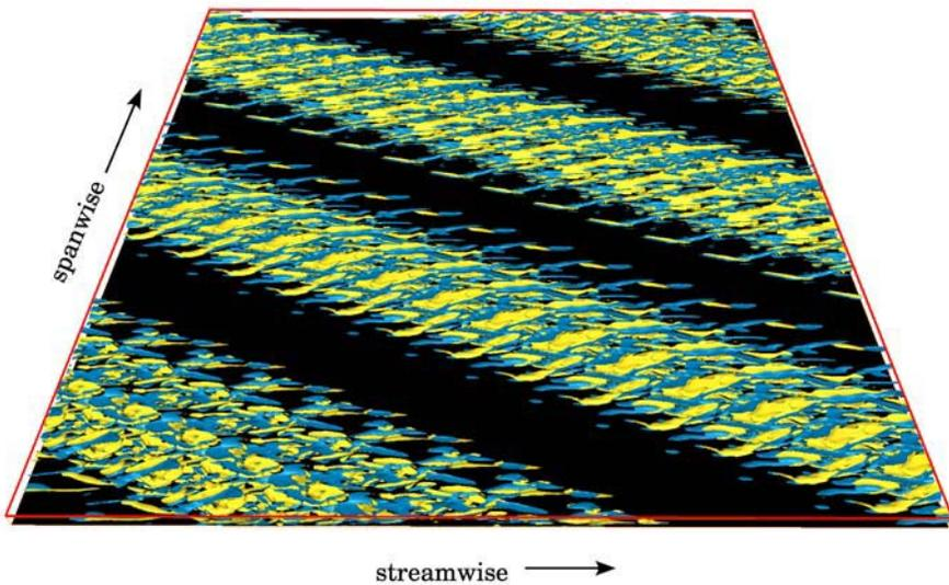
Figure 2. Turbulent-laminar pattern at Reynolds number 350. Isosurfaces of streamwise vorticity ( $\omega = \pm 0.5$ ) are shown at one instant in time. For clarity the bottom plate is shown in black while the top plate is transparent. The streamwise and spanwise extent of the region shown are 60 times the plate separation  $2h$ .
