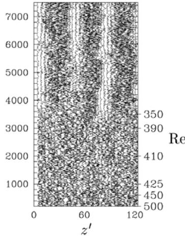
Figure 5. Space-time diagram. Kinetic energy  $E(x' = 0, y = 0, z')$  at 32 equally spaced points in  $z'$  in a domain with  $L_{x'} \times L_y \times L_{z'} = 10 \times 2 \times 120$  with tilt  $\theta = 24^\circ$ . The Reynolds number is decremented in discrete steps (right). Three long-lasting and well-separated laminar regions emerge spontaneously from uniform turbulence as  $Re$  is decreased.
