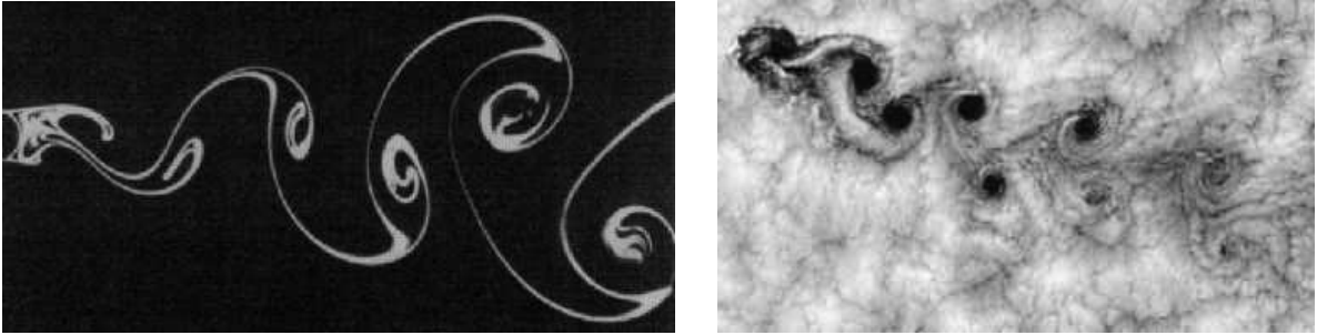
Figure 23: Von Kármán vortex street in the laboratory (left, Taneda, 1982) and in nature (right, off Chilean coast, past Juan Fernandez islands).
