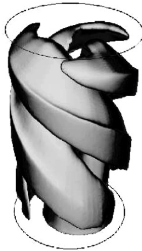
Fig. 13. Rotor–stator configuration with Re_c \approx 2150 and h = 3.5 . Isosurface u_z \approx 0 after subtraction of axisymmetric component.
