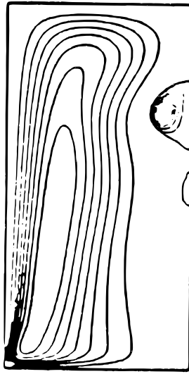
Fig. 11. Contours of Stokes poloidal streamfunction \eta from [6] for Re = 1850 , h = 2 .
