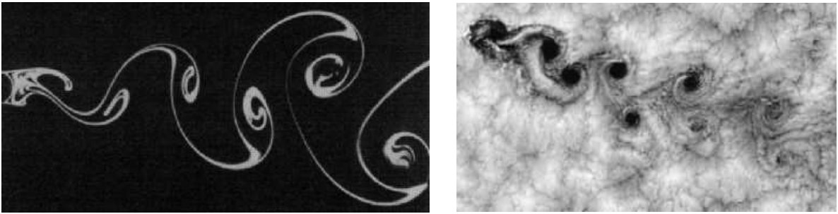
Figure 19: Von Kármán vortex street in the laboratory (left, Taneda, 1982) and in nature (right, off Chilean coast, past Juan Fernandez islands).
