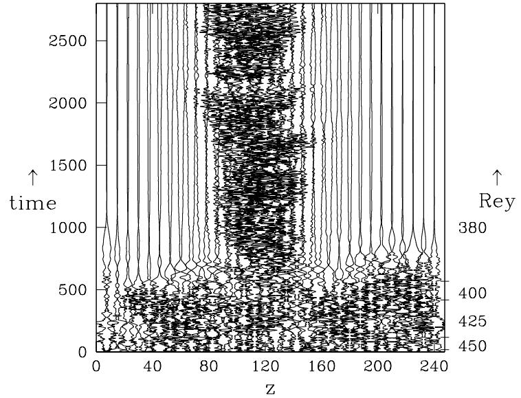
Figure 1: Space-time plot of turbulent intensity  $\|\mathbf{U} - \mathbf{U}_\parallel\|^2$  of flow perpendicular to motion of bounding plates along the line  $(x, y) = (0, 0)$  as the Reynolds number is decreased.
