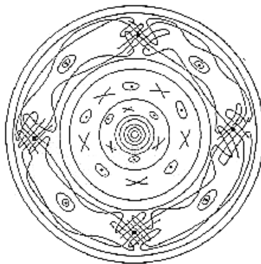
Figure 10: Non-integrable perturbation of integrable Hamiltonian system. Solid ellipses: some tori survive (those whose winding numbers are sufficiently far from any rational with small denominator). Others break into alternating elliptic and hyperbolic points. Around each elliptic point is a set of elliptical trajectories. Each hyperbolic point is surrounded by a chaotic region. From V.I. Arnol'd, Small denominators and problems of stability of motion in classical and celestial mechanics , Russian Mathematical Surveys 18:6 , 85–191 (1963). Russian version: Uspekhi Matematicheskikh Nauk. Reprinted in Hamiltonian Dynamical Systems: a reprint collection , ed. R.S. MacKay & J.D. Meiss, Adam-Hilger, 1987.
