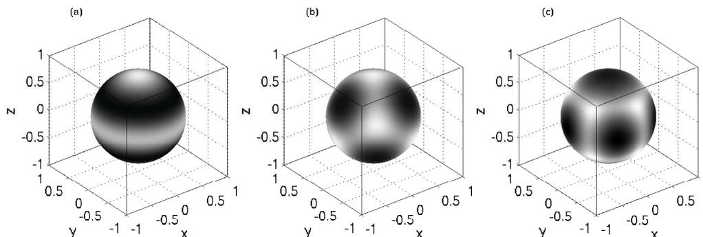
**Figure 1.** Radial velocity  $u_r$  of (a) axisymmetric state at  $Ra = 2500$ , (b) octahedral symmetric state at  $Ra = 3000$  and (c)  $m = 5$  state at  $Ra = 9000$ .
