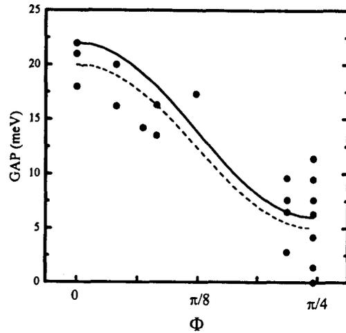
Fig. 2 : Angle-dependent calculated gap  $\Delta(\phi)$  for two sets of parameters :  $\Delta_0 = 14$  meV,  $\Delta_1 = 8$  meV, for  $T_c = 88.5$  k (solid line) and  $\Delta_0 = 12,5$  meV,  $\Delta_1 = 7,5$  meV, for  $T_c = 78.5$  k (dashed line)
