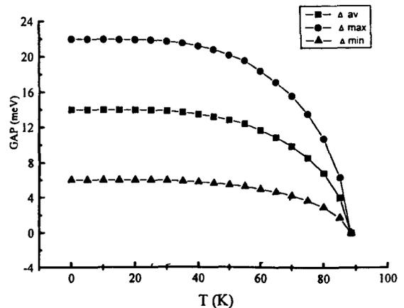
Fig. 3 : Temperature-dependent maximum (full circle), average (full square) and minimum (full triangle) gaps; for  $T = 0$  K, for  $\Delta_{\text{av}} = \Delta_0 = 14$  meV,  $\Delta_1 = 8$  meV, and for a  $T_c = 88.5$  K.
