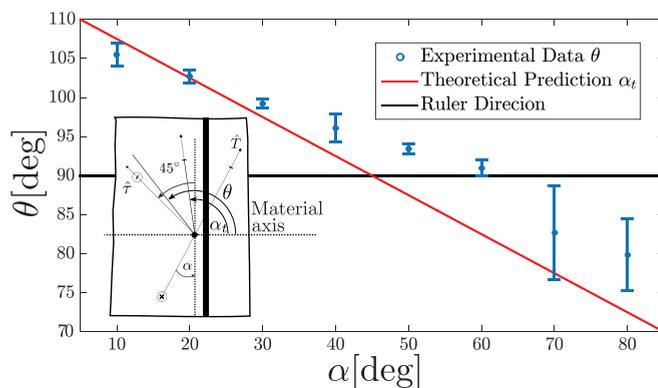
FIG. 5. Angle of fracture propagation  $\theta$  as a function of the position of the pulling point (orientation of grip vector  $\alpha$ ) for a fixed pulling angle of  $45^\circ$  with respect to the ruler. The red line indicates crack orientation as predicted by the tearing vector (3). The horizontal black line depicts the ruler orientation. Inset: Sketch of the geometry of the experiment.
