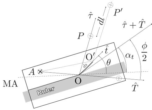
FIG. 3. Sketch depicting fracture progression. The fracture advances a distance  $ds$  following a generic angle  $\theta$ .  $dl$  is the total increment displacement of the pulling point, from  $P$  to  $P'$ , along the pulling vector  $\hat{t}$ .
