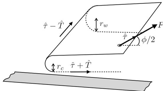
FIG. 9. Geometry of the fold as bending energy is taken into account. The fold is assumed to have a conical shape, with radii of curvature  $r_c$  and  $r_w$  at the fracture tip and at the free end, respectively.
