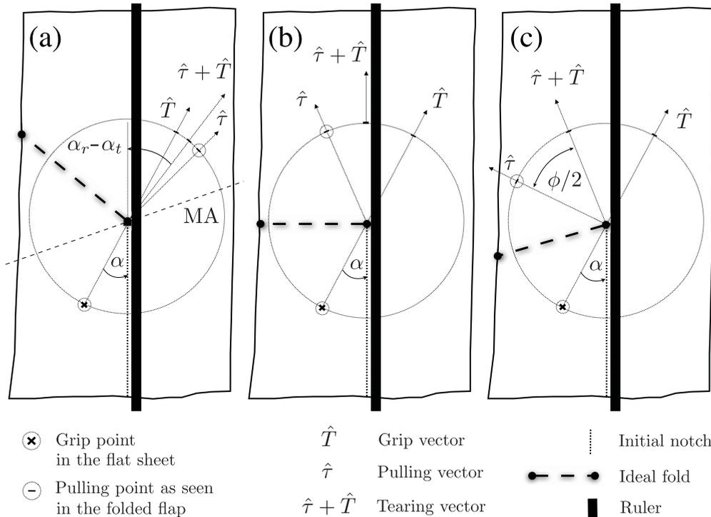
FIG. 4. Different ruler cases. (a) The tearing vector is oriented towards the ruler and the crack path follows the ruler (b) Symmetric case: the tearing vector,  $\hat{T} + \hat{t}$ , is parallel to the ruler (critical guiding). (c) The tearing vector departs from the ruler.
