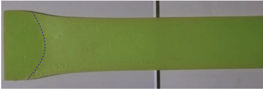
(a) Close view of the friction front emphasizing its curved shape
