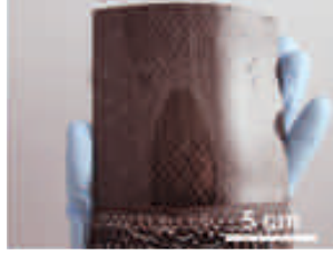
Figure 3.2.: Adhesive pad composed of a stiff fabric imbibed with a soft adhesive elastomer, image extracted from [60].
