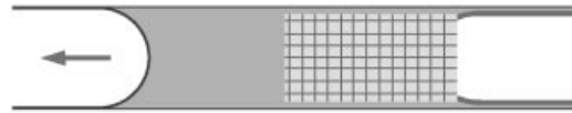
FIGURE 29. Running gel: a gel composed of a mixture of cross-linking silicone and inert silicone oil is juxtaposed to a first index of ethylene glycol. The observed spontaneous motion relies on the extraction of a film of silicone oil from the gel.
