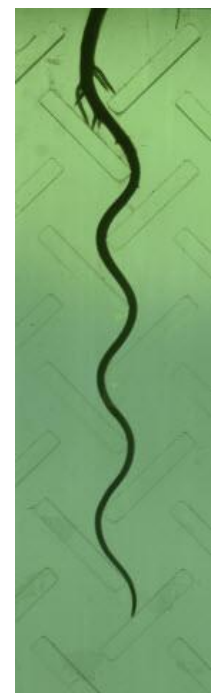
Chick-pea root growing in hydroponics in an assembly of circular posts of PDMS (top left) or 3D-printing polymer arrays of baffles (bottom left: design; right panel: experiment)
