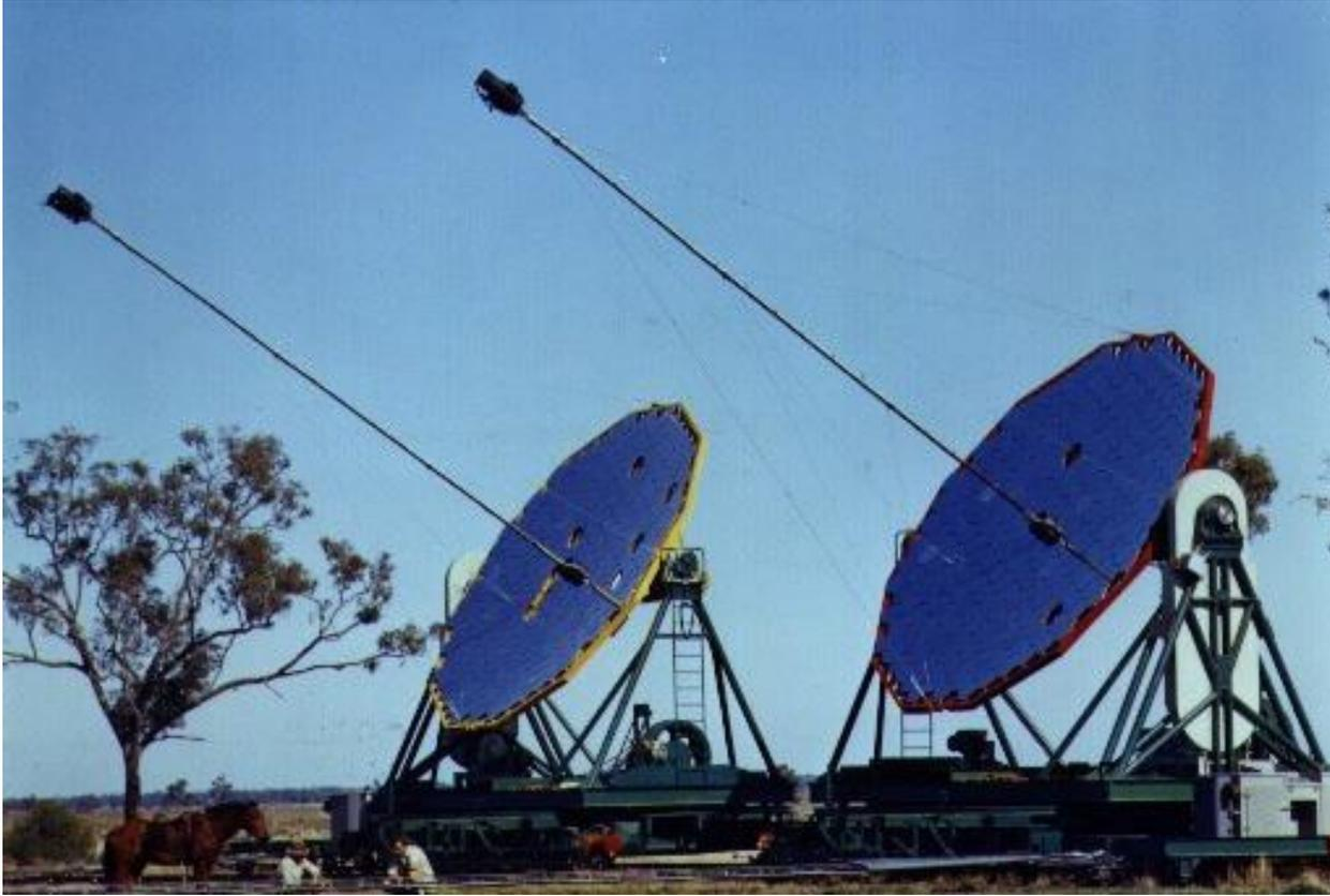
The hanbury brown-twiss intensity interferometer at narrabri, new south wales, Australia
