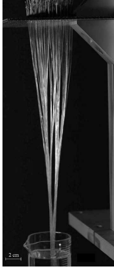
Fig. 1: Brush of fibers withdrawn from a bath of silicon oil. The brush is made of 100 optical fibers with 0.4 mm diameter, spaced by 3.1 mm.
