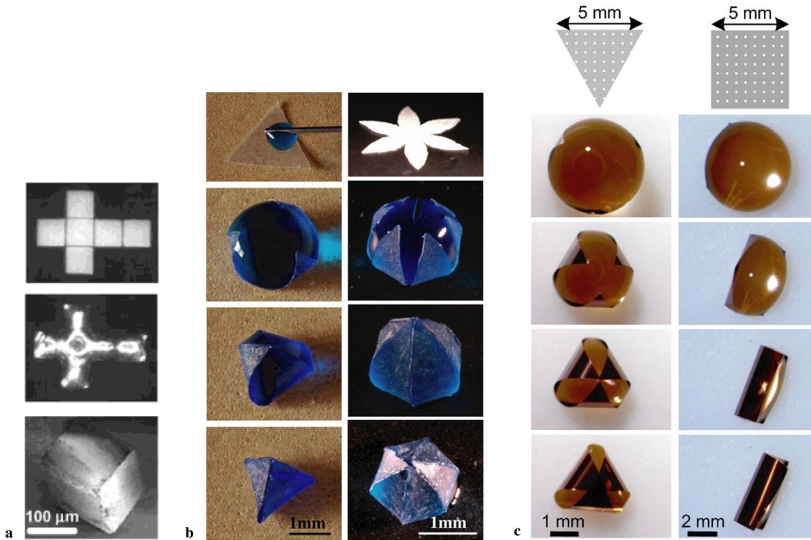
**Figure 10.** (a) Capillary ‘origami’. Closing of hinged structures inside a liquid droplet [107] (molten solder on metal templates). Copyright Wiley-VCH Verlag GmbH & Co. KGaA. Reproduced with permission. (b) and (c) Self-wrapping of a flexible sheet (PDMS and silicon) around a droplet of water leading to different 3D structures depending on the initial template, images reprinted from [58] and [116], respectively, with permission.
