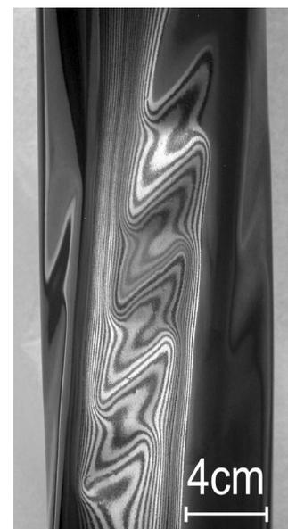
FIG. 3. Initial buckling pattern on the cylinder under torsion
