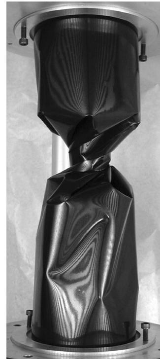
FIG. 6. Secondary S structure after locking of the primary pattern. There is a hierarchical cascade of S-structure formation for increasing torsion.
