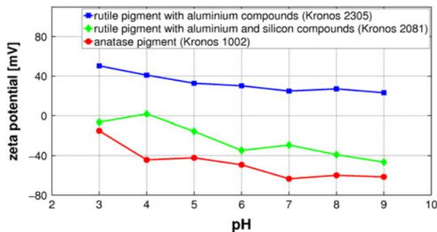
Fig. 2 Zeta potential as a function of  $\text{pH}$
