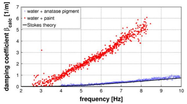
**Fig. 8** Absolute damping coefficient  $\beta_{\text{calc}}$  in the function of the frequency. Comparison of the water suspensions obtained by adding anatase pigment and white paint. The *black line* is the theoretical attenuation  $\beta_0$  given by Stokes (Eq. 5)
