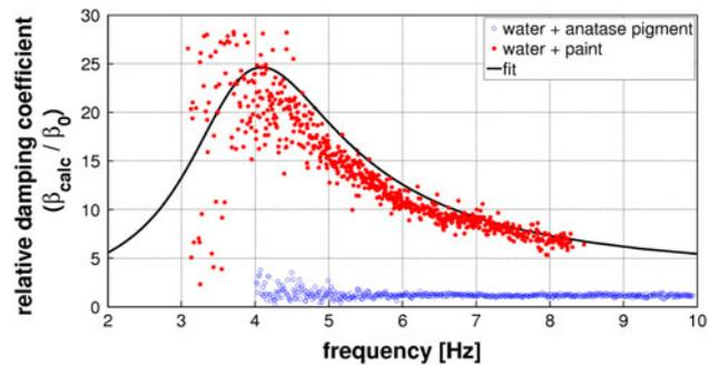
**Fig. 9** Relative damping coefficient ( $\beta_{\text{calc}}/\beta_0$ ) in the function of the frequency. Comparison of the water suspensions obtained by adding anatase pigment and white paint. The *black line* is the theoretical fit based on the formula proposed by Alpers (1989)
