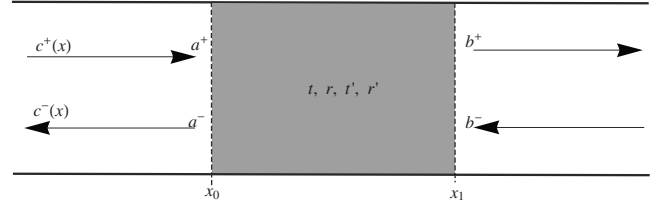
FIG. 6. Illustration of a quasi-one-dimensional waveguide composed of one unit cell (gray) connected to two ideal leads going to infinity. The field [Eq. (17)] at the unit cell's boundaries is given by [c_i^+(x_0) \ c_i^-(x_0)] = [a_i^+ \ a_i^-] and [c_i^+(x_1) \ c_i^-(x_1)] = [b_i^+ \ b_i^-] . Solving the scattering problem in this geometry we can obtain the Bloch basis of the infinite periodic chain.
